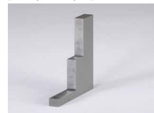
Die steel, 10-50-100mm 1 rough, 3 skims Accuracy \pm 3.0\mu\text{m} R_z 3.3\mu\text{m} ( R_a 0.36\mu\text{m} )
