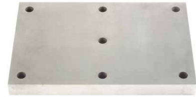
Die steel, 25mm 1 rough, 5 skims Pitch accuracy -1.2\mu\text{m} to +1.0\mu\text{m}
