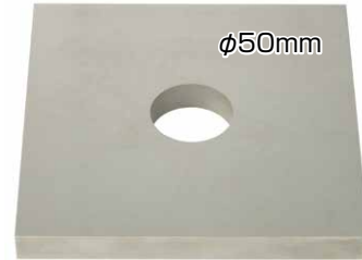
Die steel, 20mm 1 rough, 5 skims Roundness 0.90\mu\text{m}
