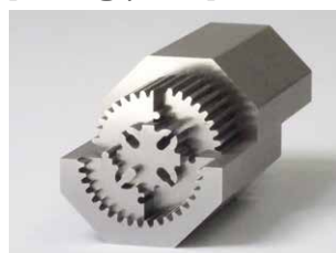
Die steel, 40mm 1 rough, 3 skims Accuracy \pm 3.0\mu\text{m} R_z 2.5\mu\text{m} ( R_a 0.30\mu\text{m} )
