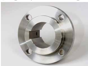
Stainless, 40mm 1 rough, 1 skim Accuracy \pm 5.0\mu\text{m} Cutting speed 13% faster
